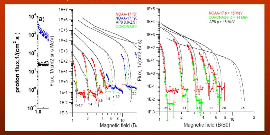
Low energy trapped protons fluxes measured by considered satellites are underestimated by the model at L< 1.4-1.6 coincide with the model at L~1.8 and overestimated by the AP8 model at L>1.8.
