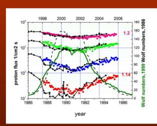
Trapped proton flux at geomagnetic equator for several L-shells observed in 21-23 solar cycle WRMISS 13 Kraków, Poland September 8-10, 2008
