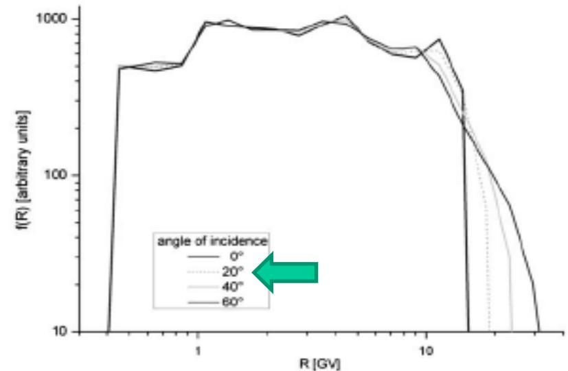
Fig. 2. Cut-off distribution for different angles of incidence for a telescope pointing towards the geographical zenith direction.
