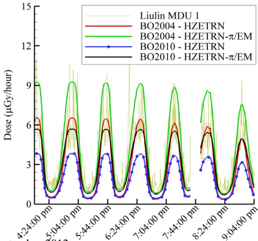
Comparison of models to measured data taken aboard ISS on July 6, 2001
