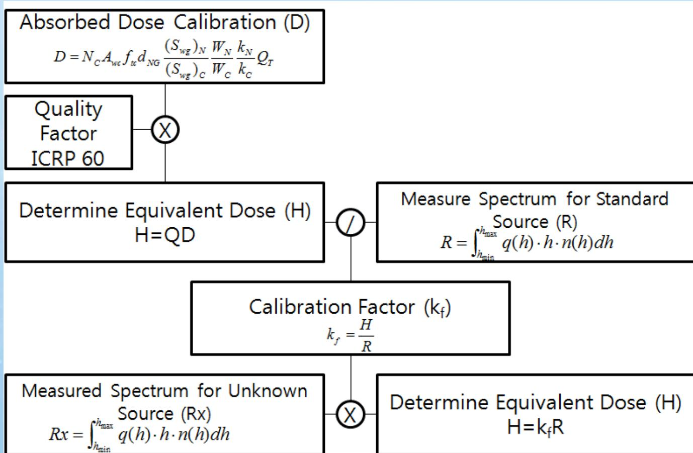
Process of Equivalent Dose Calibration
