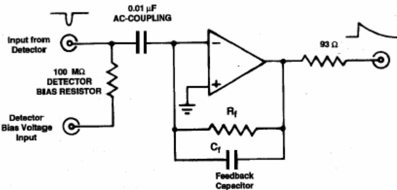
Fig. 6.1. Typical RC feedback charge sensitive preamp.
