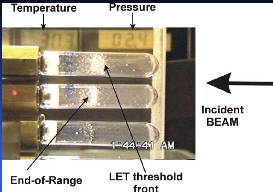
$$\text{Super Heat: } S = \frac{T - T_b}{T_c - T_b}$$
