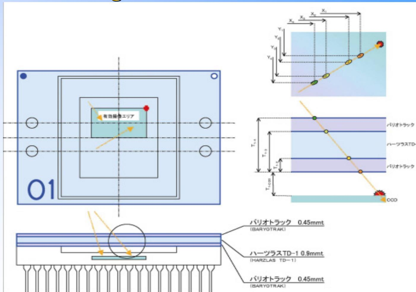
HZE particles penetrate to the effective area of CCD elements
