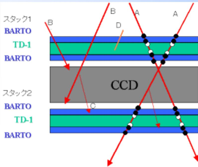
**Arrangement of CCD elements
