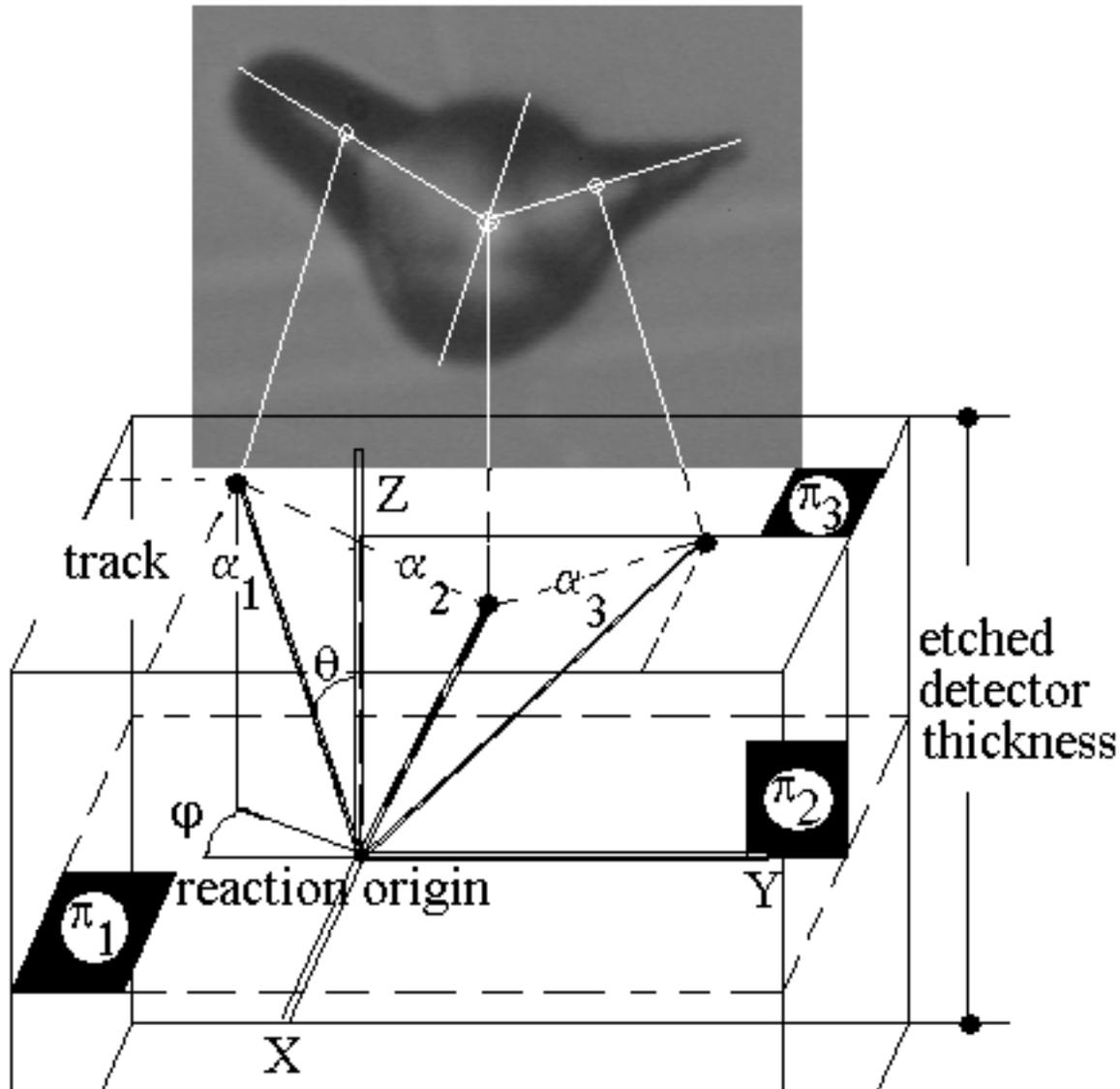
In plane  $\pi_3$  we estimate the position of the latent track and from the digitalized image we deduce the geometry of the track mouth. The shape usually is the superposition of three ellipses having different eccentricity. The measured parameters allow us to determine, in principle, the direction and the range (energy) of the particles.
