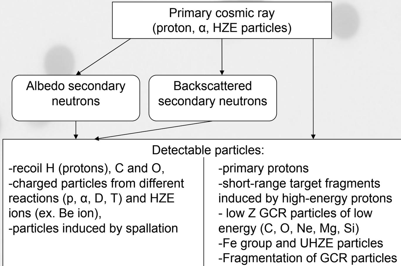
Particles induced by primary cosmic rays and secondary neutron radiation which can be detected in the space on the **PADC sheets**
