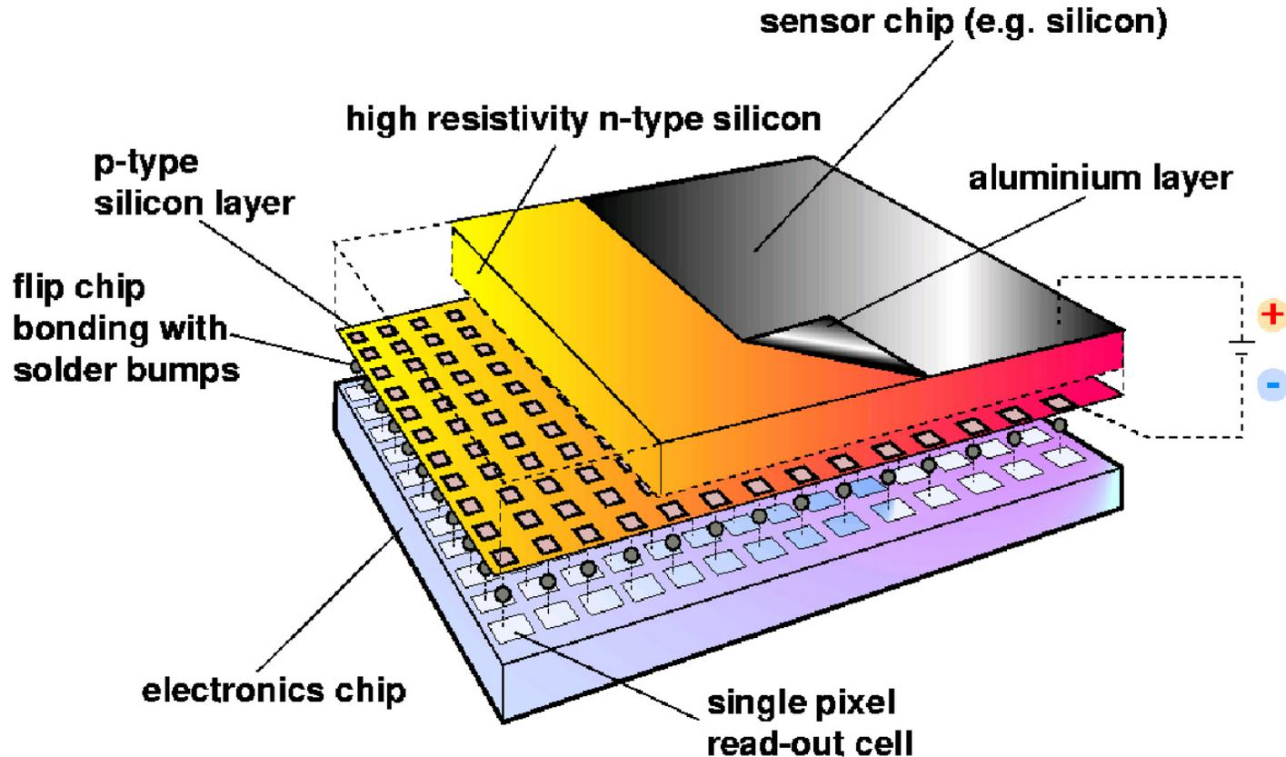
**Detector and electronics readout are optimized separately**
