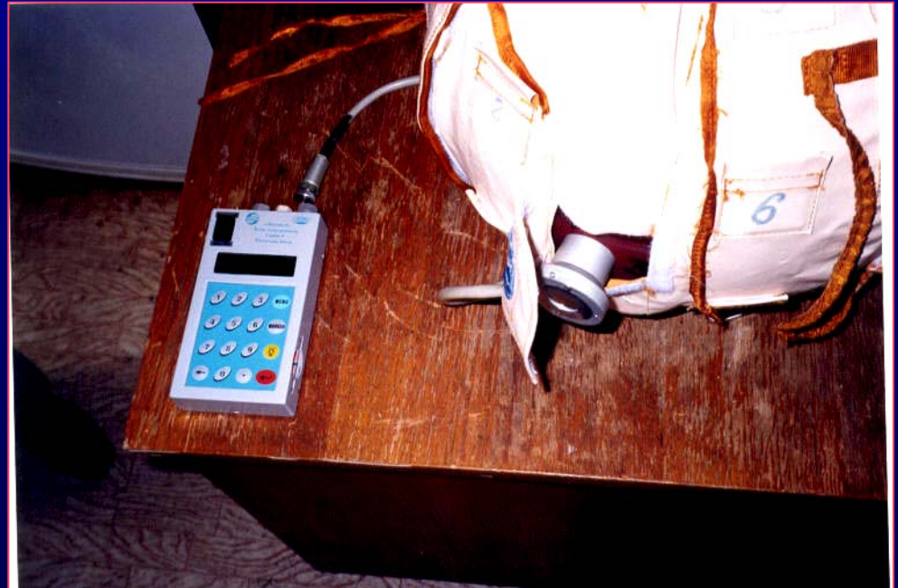
Liulin-5 in the spherical phantom
