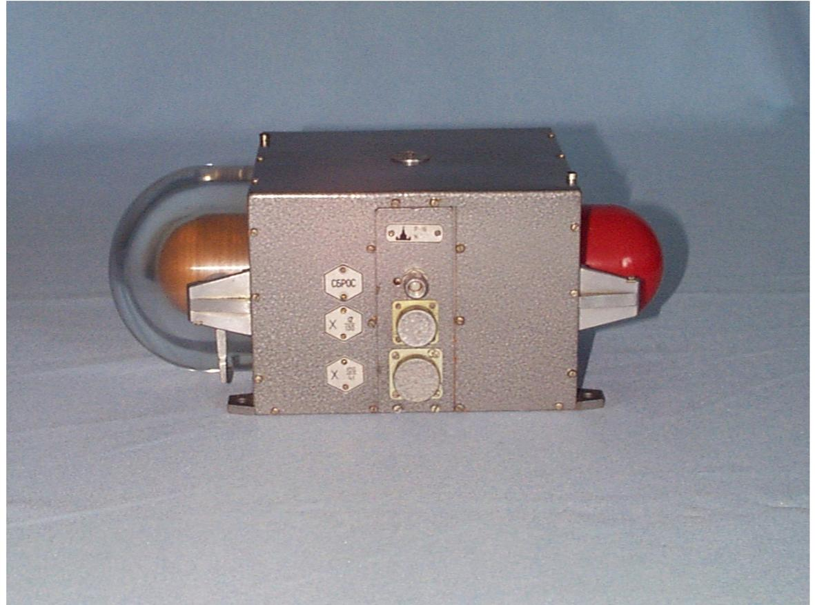
**Pulses from ionisation chambers are counted up. The number of the pulses is transferred directly to the telemetry system of RS ISS.**
