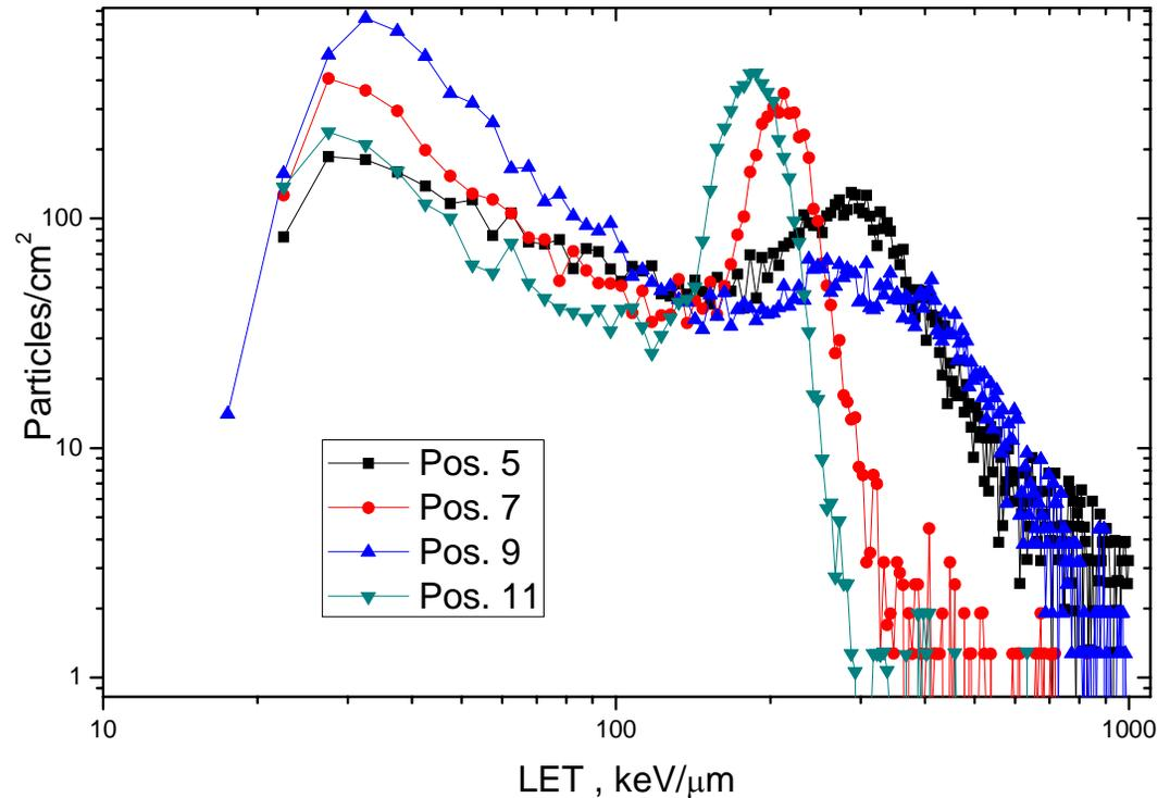
Low LET particles ( $<100 \text{ keV}/\mu\text{m}$ ) are slowed down carbon ions while the higher ones ( $> 300 \text{ keV}/\mu\text{m}$ ) were induced by He ions via target fragmentation procedure. The distinct peaks can be related to the Fe ions.
