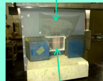
Laser pointing to center the samples
