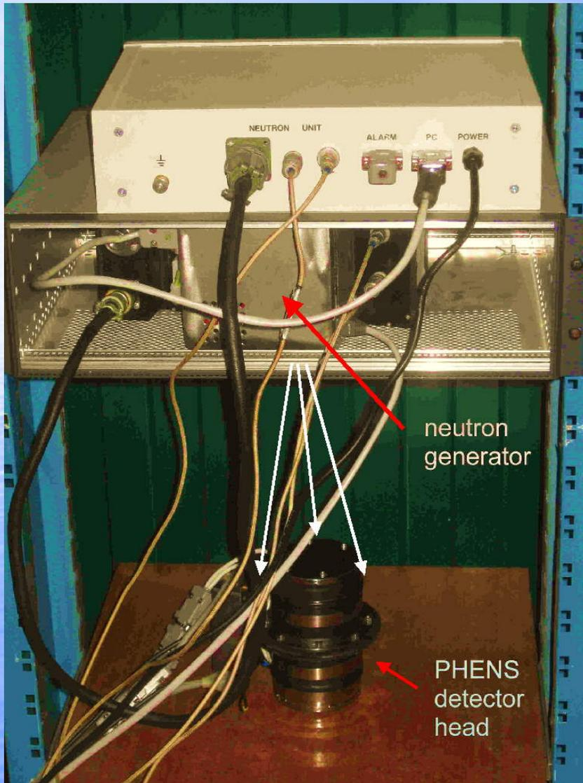
First calibration measurements at 14 MeV neutrons were performed using a D-T neutron generator. Neutron flux intensity was about  $7 \times 10^7 \text{ s}^{-1}$  in  $4\pi$ .
