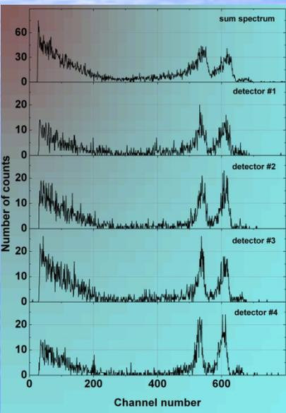
**Four internal  $^{238}\text{U}$   $\alpha$ -particle sources (6 Bq each) provide checks of operationability and gain stability and energy calibration**
