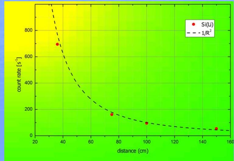
Neutron flux was measured by means of the generator internal counter of accompanying  $\alpha$ -particles and external monitor based on  $^{238}\text{U}(n,f)$  reaction.
