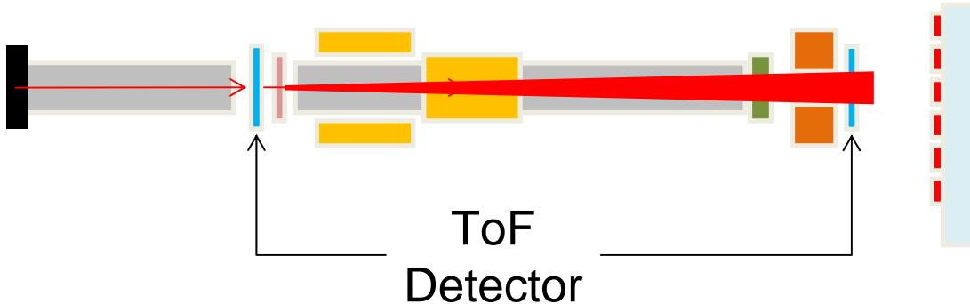
We have measured the energy of the beam by means of ToF (Time of Flight)
