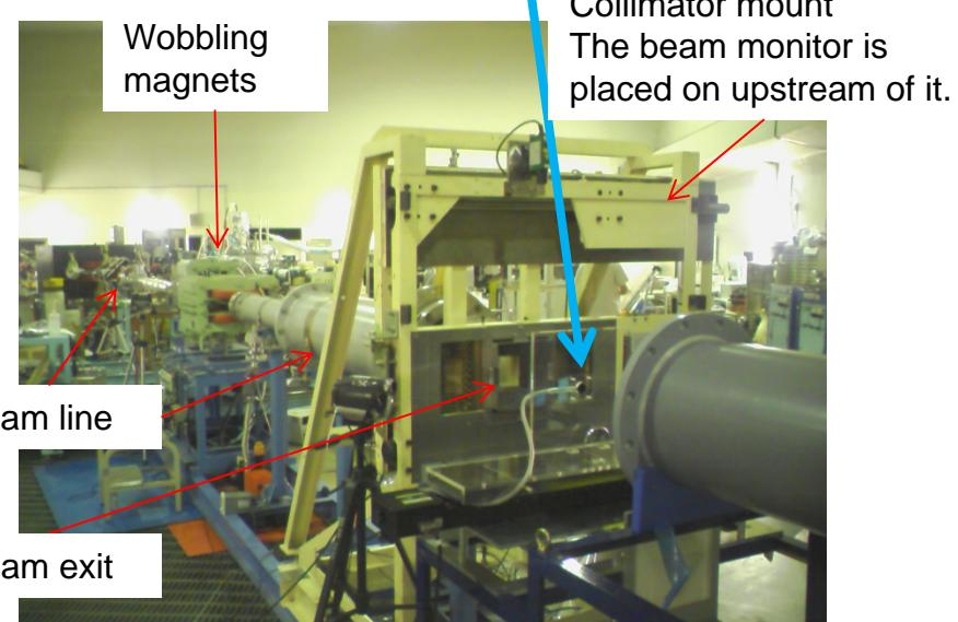
Calibration of the beam monitor
