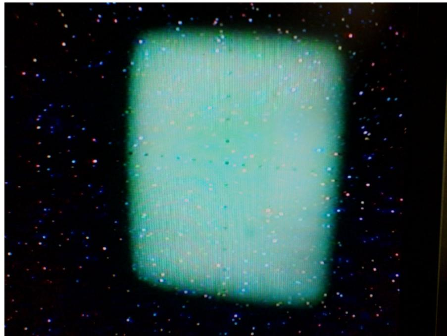
Photo of the beam image using a luminescence plate.
