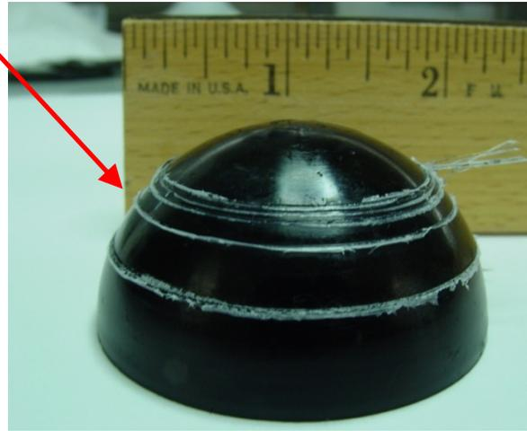
Development of spherical TEPC detectors to replace cylindrical detectors currently onboard ISS
