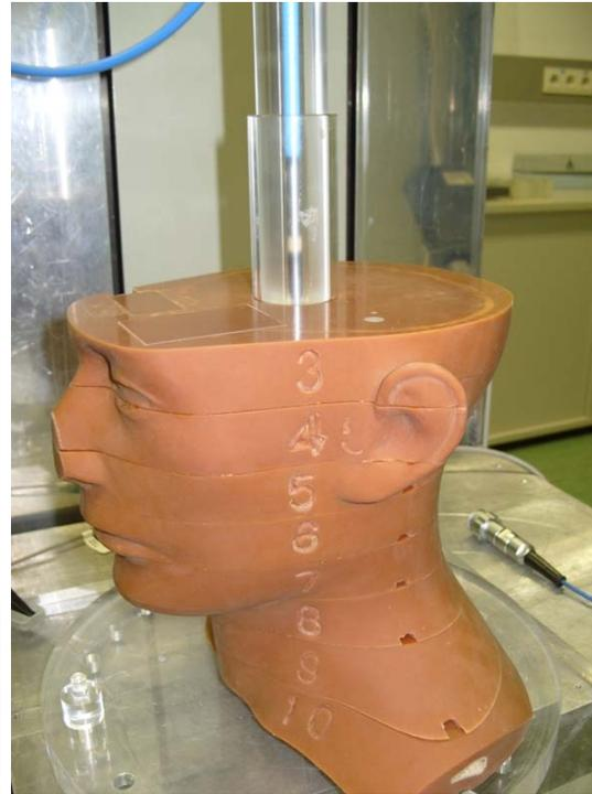
Chamber in PMMA rod , slice #2
