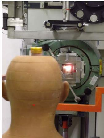
MATROSHKA head in front of the irradiation facility, reference point is marked
