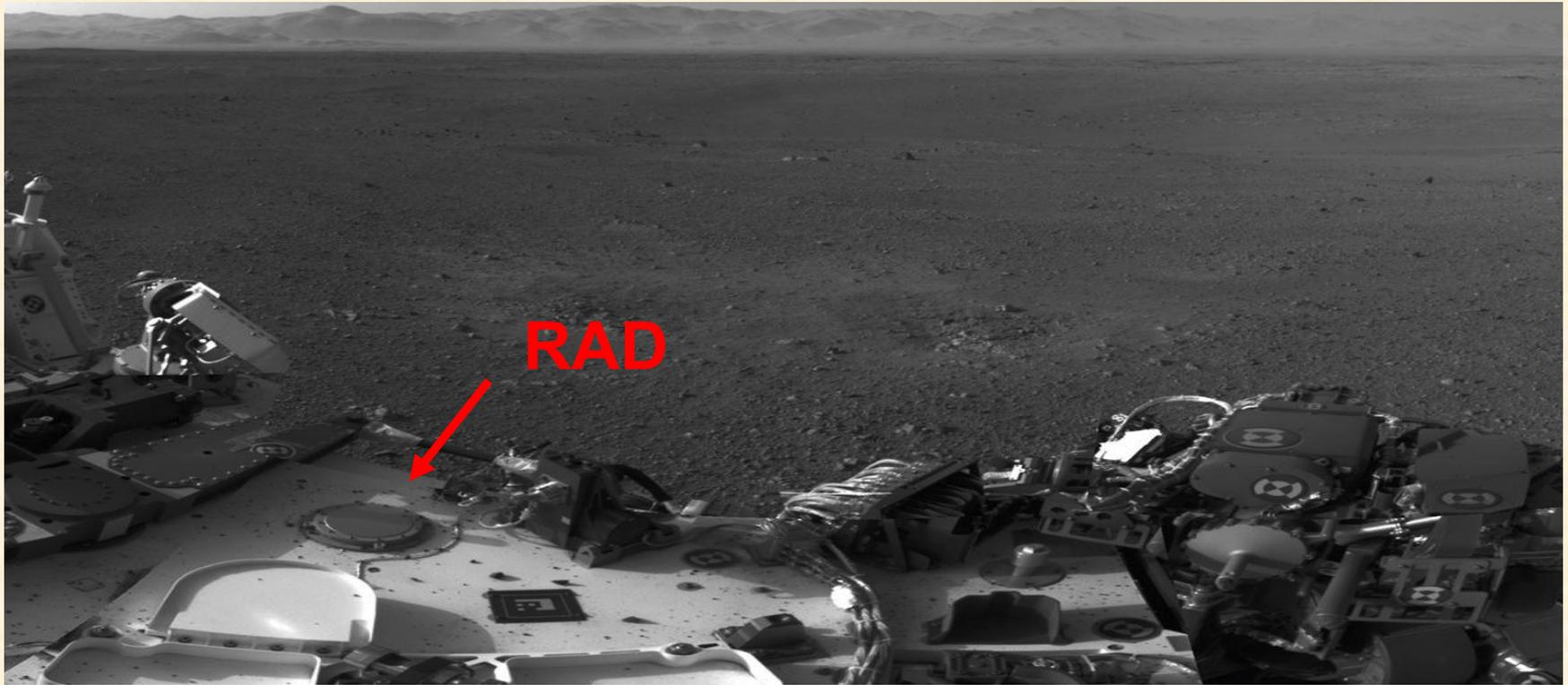
The Curiosity rover successfully landed in Gale crater on August 6, 2012. Situated on board the rover, RAD is the first-ever instrument to measure the Martian surface radiation environment.
