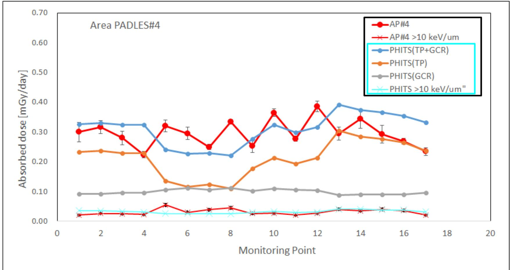
Comparison between Area PADLES#4 measurement and PHITS calculations in exact geometry of Kibo(ISS)
