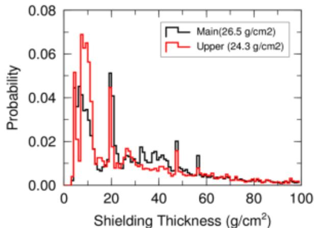
Shielding distribution from center of the KIBO
