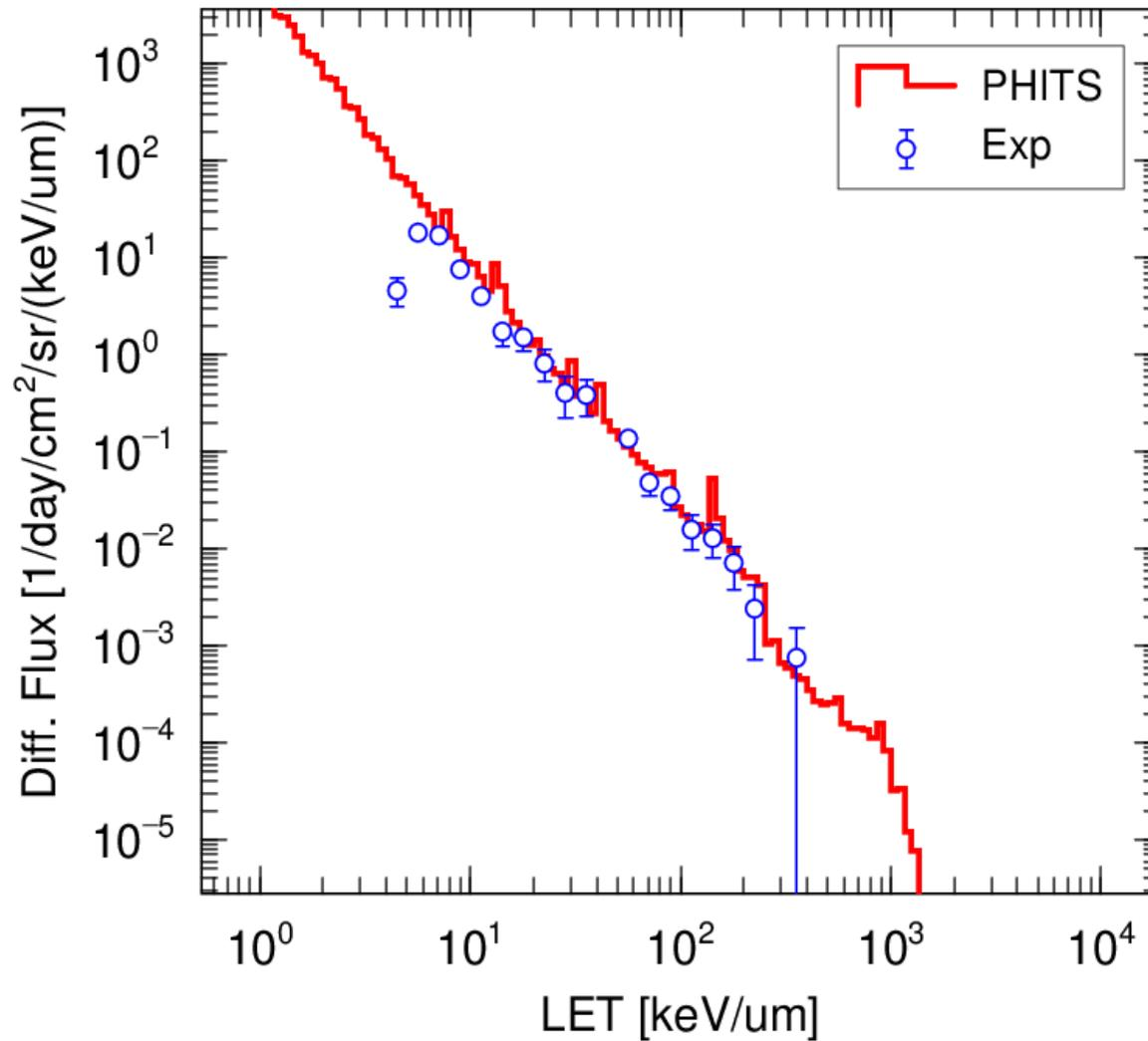
The LET distributions (in monitoring point 1) measured in the Area PALDES #4 experiment are compared to results of PHITS calculations using a well developed shielding model of the KIBO.
