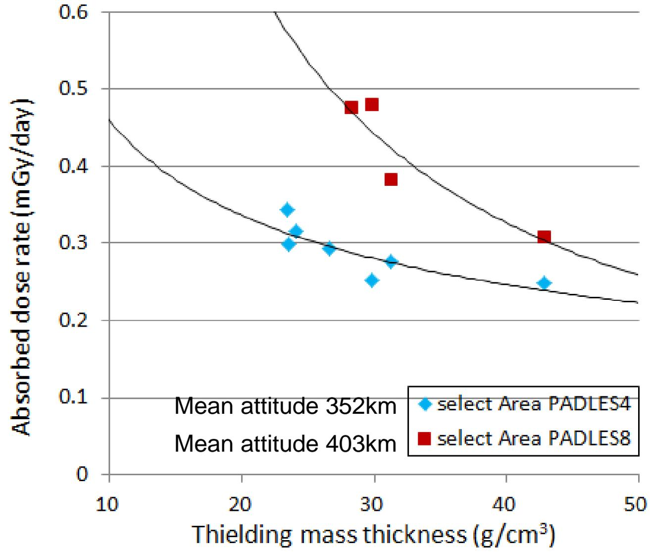
Shielding mass thickness of 17 Area PADLES monitoring points are in the 22.2 to 50.3 g/cm² range.
