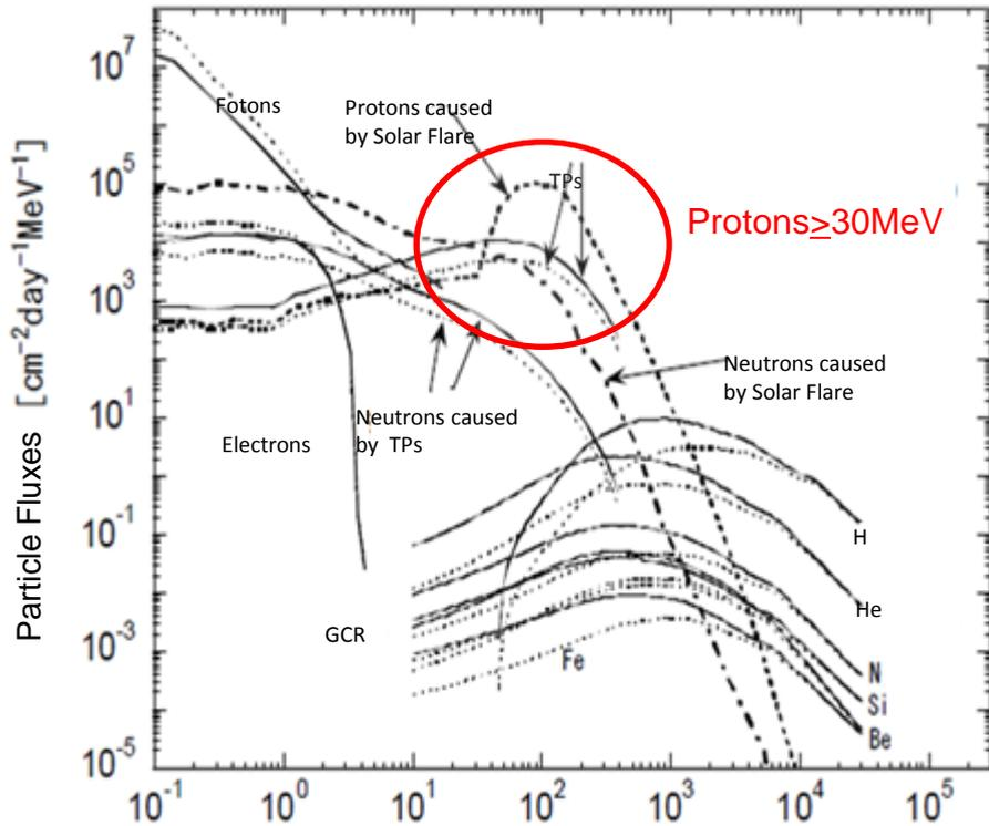
Particle Fluxes of various space radiation particles inside the ISS at an Attitude of 407.44km, the inclination of orbit is 51.6 degrees. The ISS module hull has an 9.5mm thick film of aluminum.
