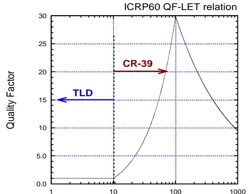
CR-39 measures a LET distribution of particle fluence  $\geq 10 \text{ keV} / \mu\text{m}$
