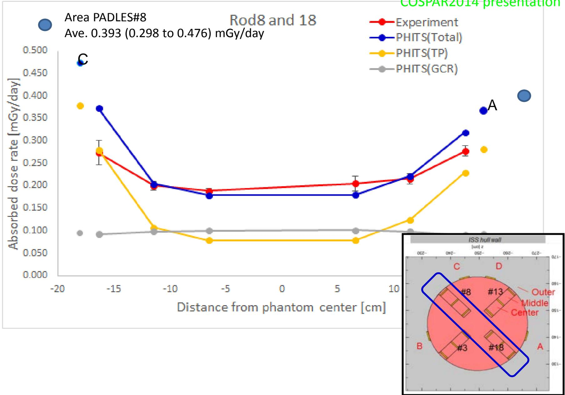
Pleliminary attemp: Distance from ISS KIBO Hull to maeasurement point in both Matroshka experiment
