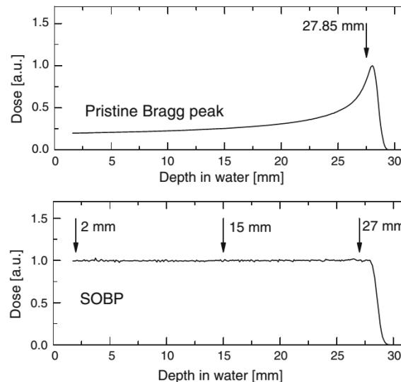
**Fig. 1** Depth-dose distributions of the proton beam produced at the IFJ PAN Kraków (nominal energy 60 MeV) measured in a water phantom using a Marcus ion chamber. *Upper panel:* pristine beam; *lower panel:* SOBP. Arrows indicate positions at which cells (human fibroblasts) were irradiated: near (at 27.85 mm) the maximum of the Bragg peak in a pristine beam, and at three depths (2, 15, and 27 mm) of the SOBP of full width 28.4 mm
