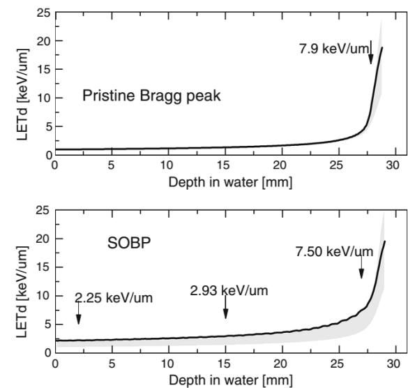
**Fig. 2** Depth distributions of dose-averaged LET ( $LET_d$ ) and of IQR of  $LET_d$  (shaded) of the proton beam produced at the IFJ PAN, simulated by Monte Carlo calculations. *Upper panel:* pristine beam; *lower panel:* SOBP. Calculated values of  $LET_d$  at irradiation positions are also shown
