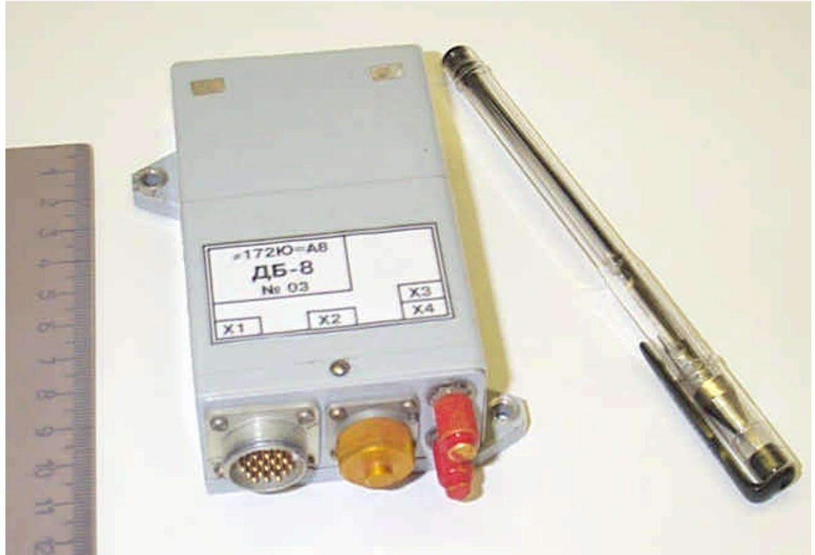
The sensitive component is a silicon semiconductor detector of 300 mm sensitive layer covering an area of 1 cm<sup>2</sup>.
