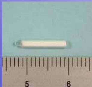
$\text{Mg}_2\text{SiO}_4 : \text{Tb}$  powder enclosed
