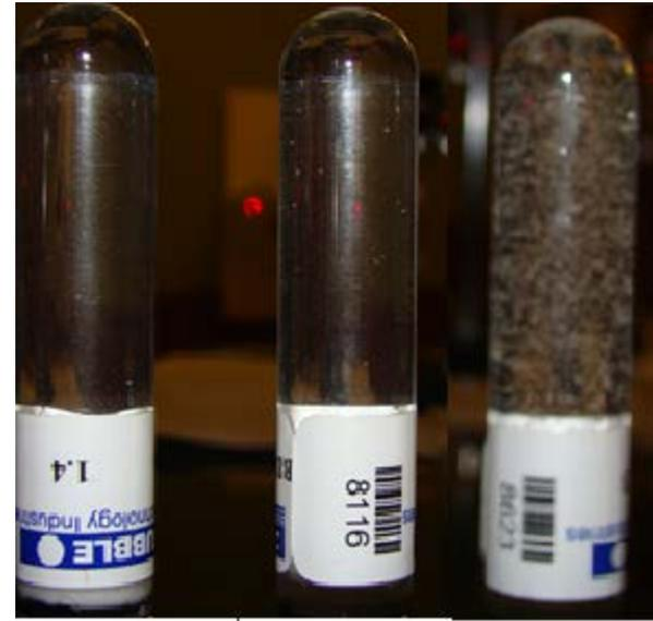
Three bubble detectors after irradiation with 78.2 MeV proton beam
