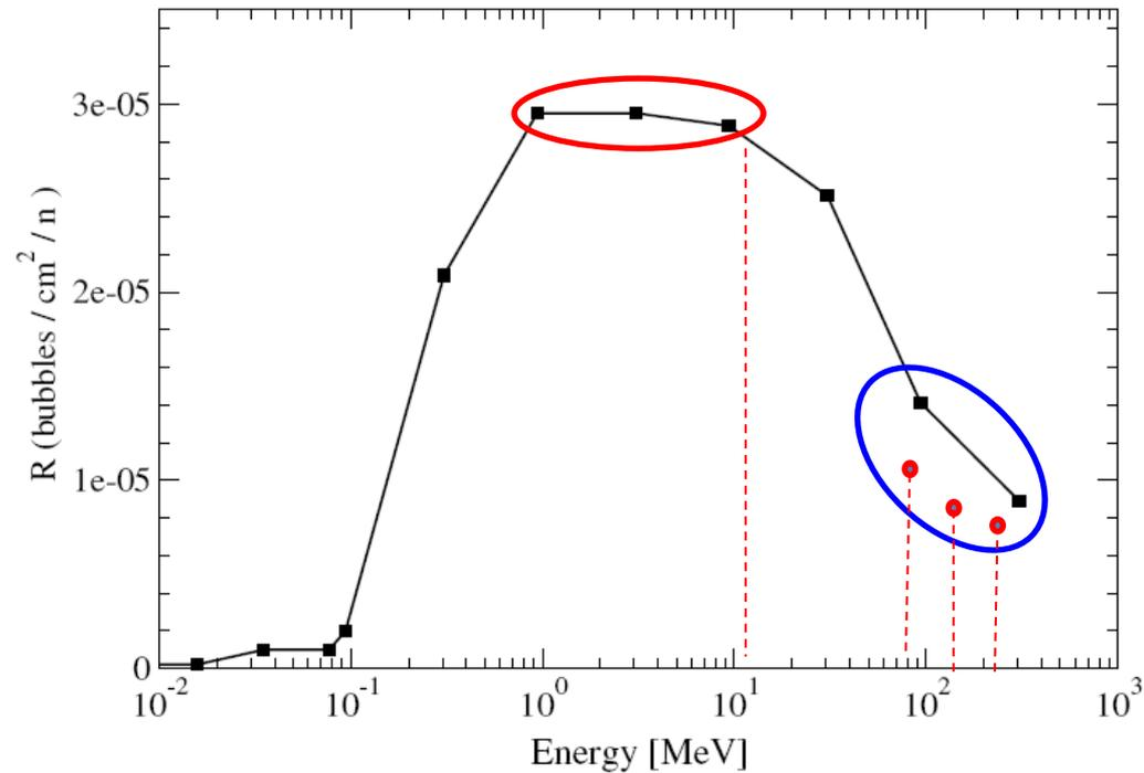
**Figure 13:** Response of bubble detector to neutrons [5]
