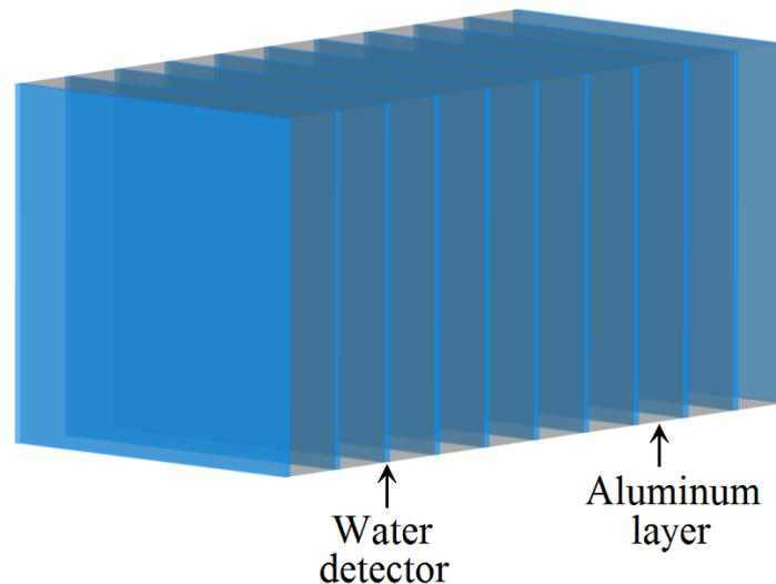
Geometry setup for Monte Carlo calculations (not to scale).
