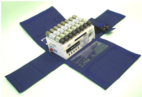
With the system consisting of a lightweight reader device and a number of TL dosimeters, more than 30 000 read-outs were carried out until now. The Pille system provides monthly dose data from locations of the space station including Matroshka while two dosimeters are dedicated to EVA measurements, and
