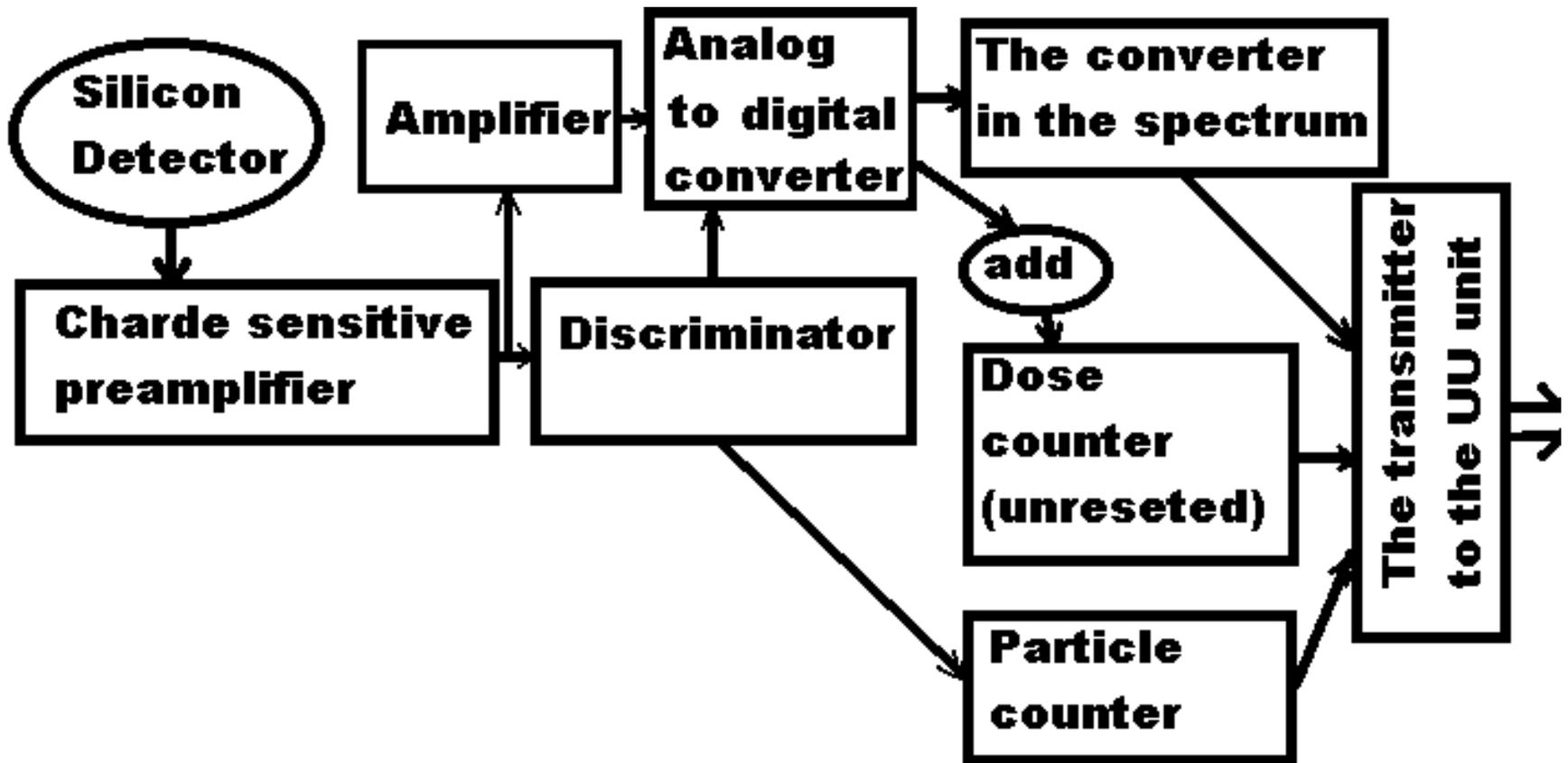
**If we neglect the system noise and round off errors then the absorbed dose is proportional to the sum of the ADC output signal.**
