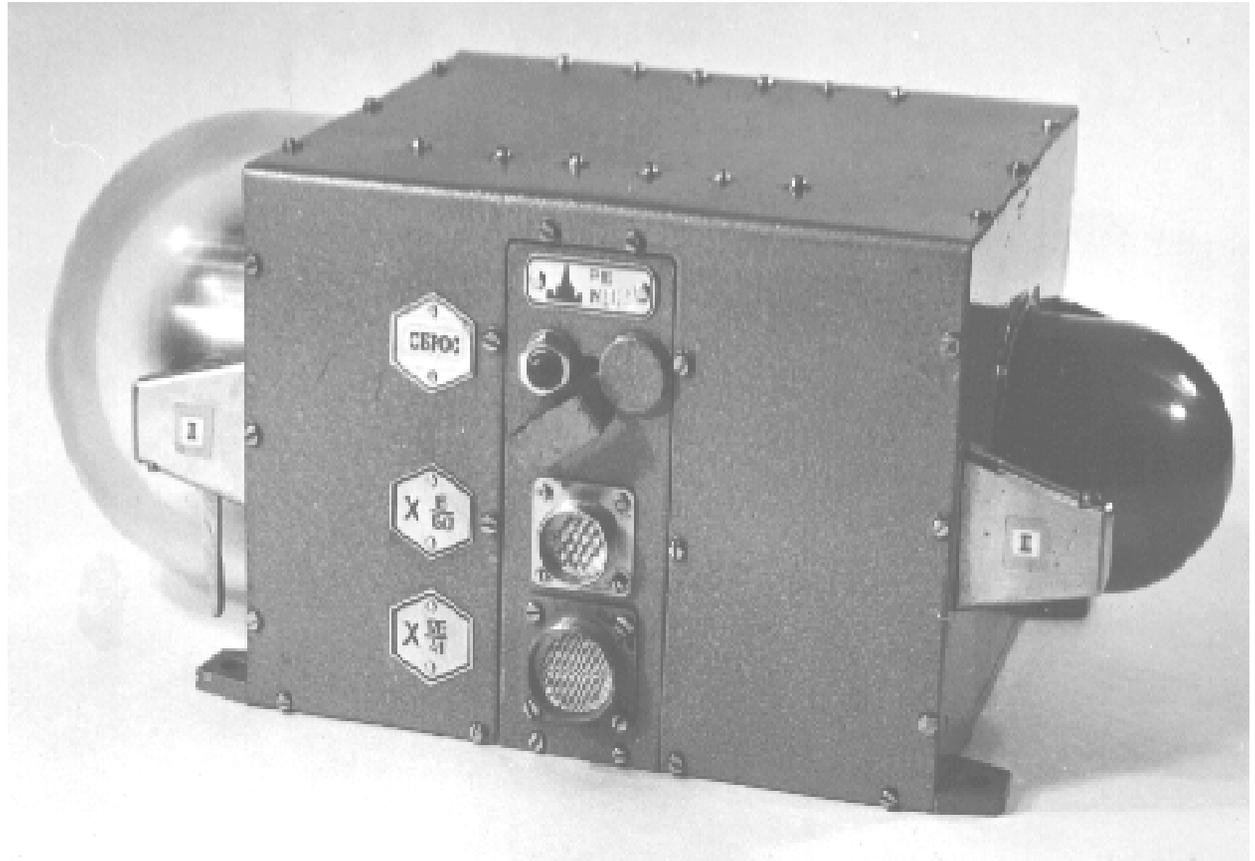
Pulses from ionisation chambers are counted up. The number of the pulses is transferred directly to the telemetry system of RS ISS.
