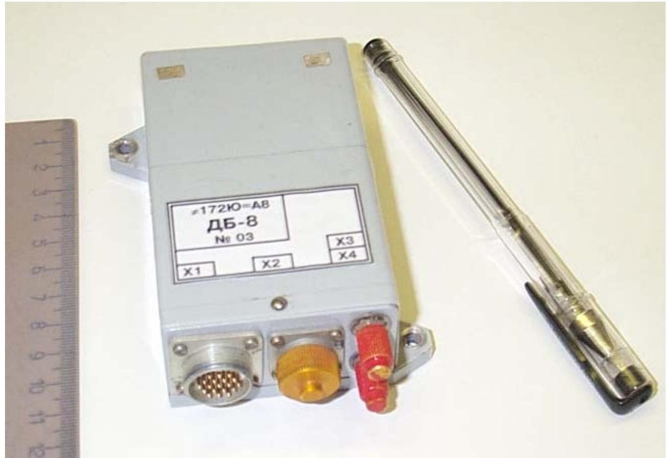
The sensitive component is a silicon semiconductor detector of  $300 \mu\text{m}$  sensitive layer covering an area of  $1 \text{ cm}^2$ .
