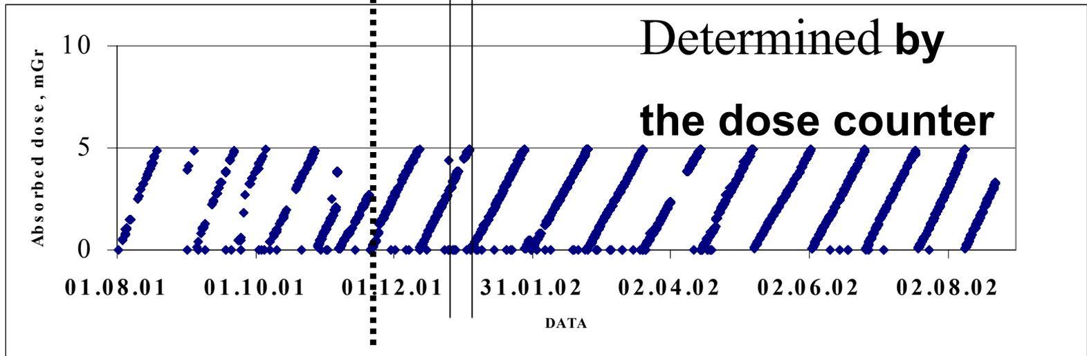
**The data given on the previous slide illustrate monotonous increase of the absorbed dose; at some moments the increase is interrupted and dose value restarts the increase from zero (dose resets).**
