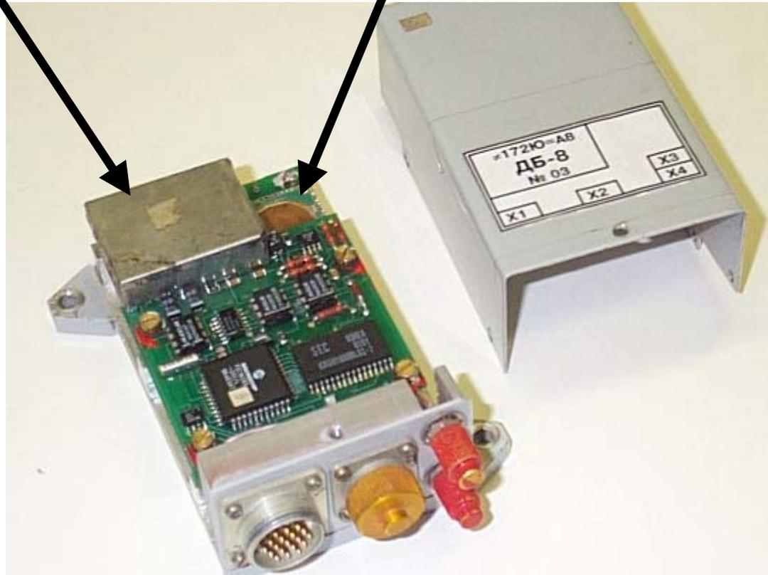
Each DB-8 unit consists of 2 independent dosimeters
