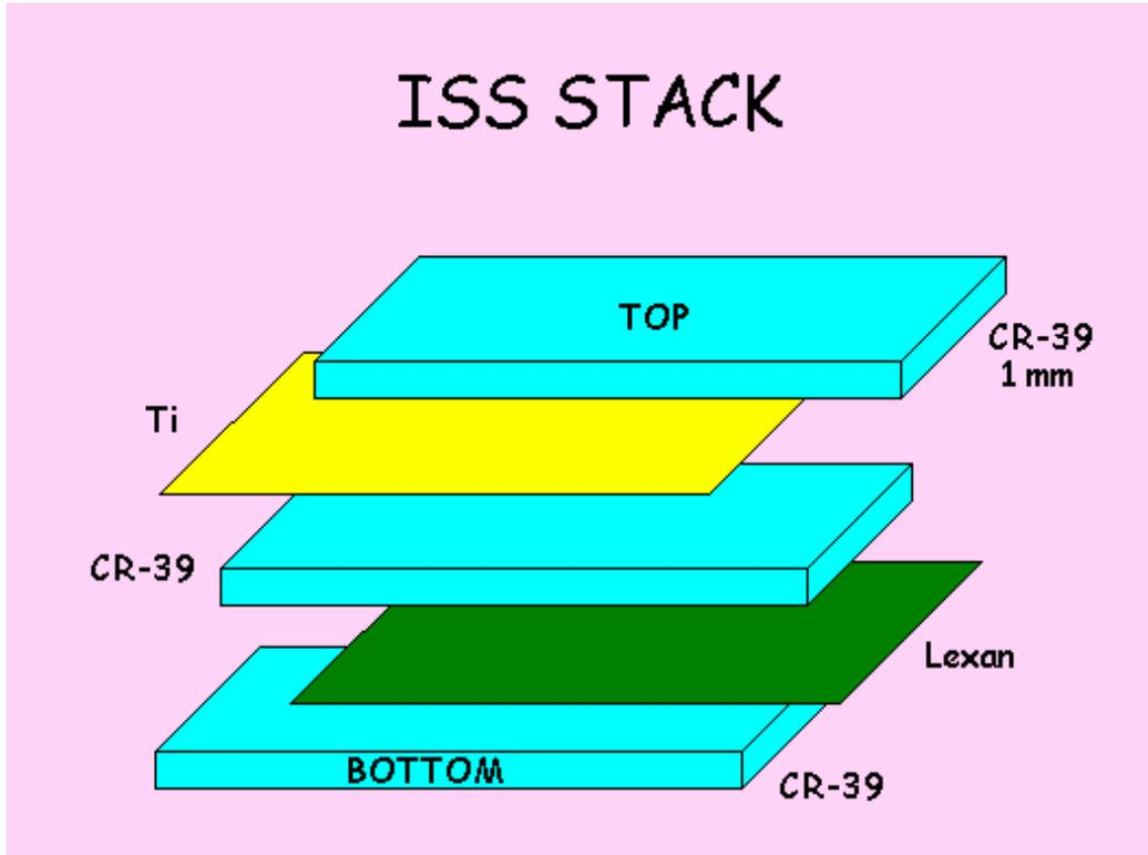
Fig. 1. Track detector assembly (stack) developed to determine the neutron dose on the ISS.
