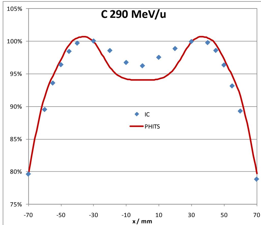
PHITS simulation: transverse dose distribution at the front surface of water column
