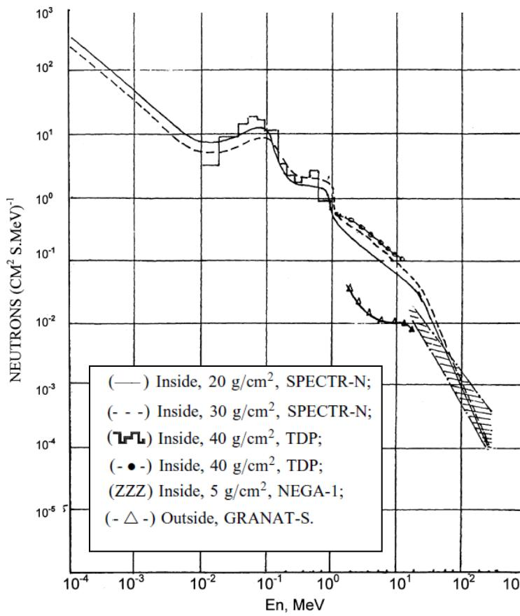
*Neutron spectra inside and outside Mir station measured with different instruments, V. I. Lyagushin, V.E. Dudkun et al., Radiation Measurements, 33 (2001), 313-319*
