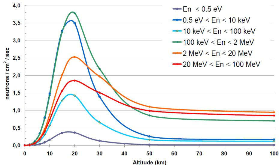
Total flux of neutrons for all energy crossing the surfaces at specified amplitudes
