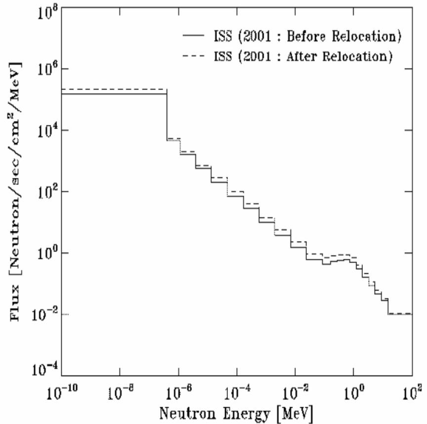
*Evaluation of neutron radiation environment inside the ISS based on Bonner Ball Neutron Detector Experiment (H. Koshiishi, H. Matsumoto, et al., Proc. 9<sup>th</sup> WRMISS, 2001)*
