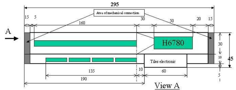
Dimensions of the scintillation counter and SiPM tiles:  $295 \times 124 \times 45 \text{ mm}^3$
