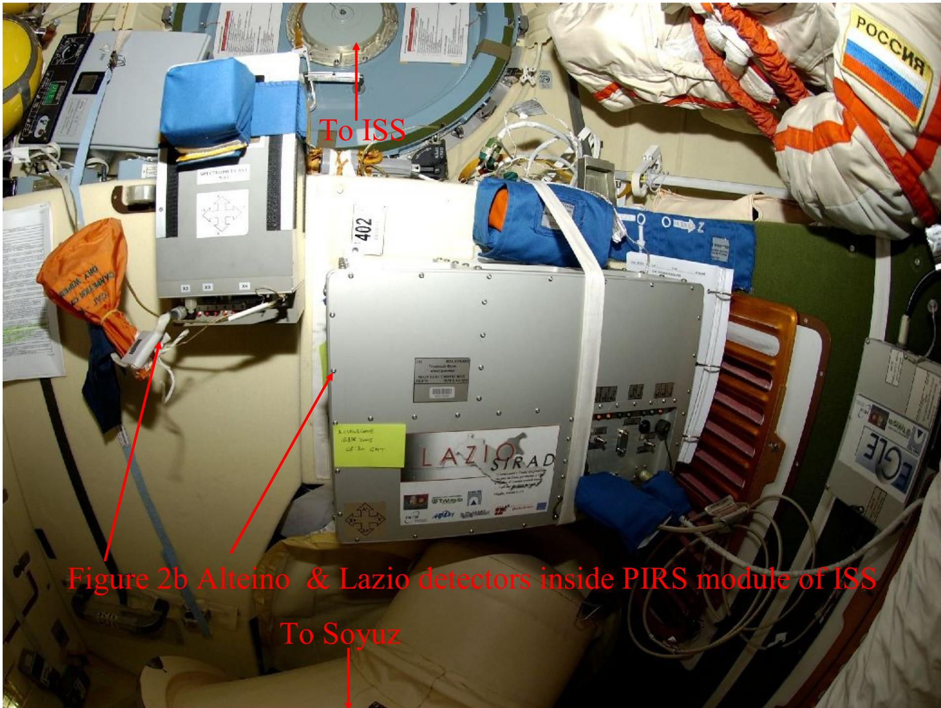
Figure 2b Alteino & Lazio detectors inside PIRS module of ISS
