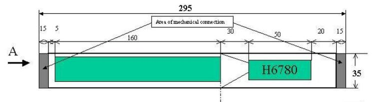
Dimensions of the scintillation counter Sc2:  $295 \times 124 \times 35 \text{ mm}^3$
