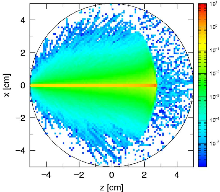
**Dose** Distribution in Tissue Equivalent Material Irradiated by 100 MeV Proton
