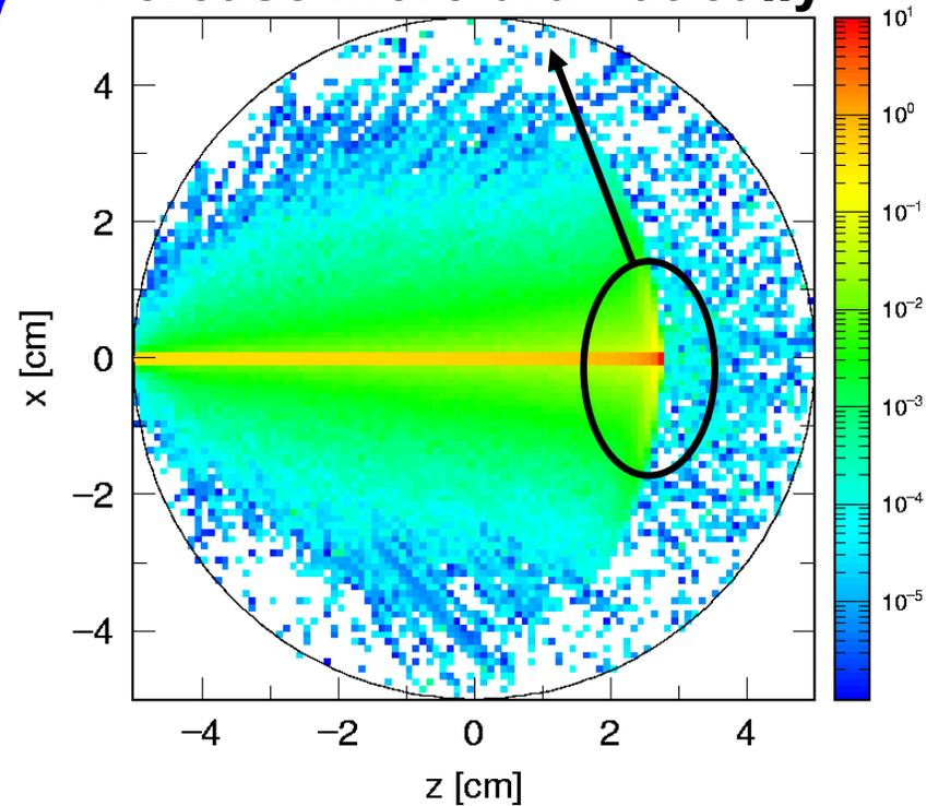
**Dose Equivalent** Distribution in Tissue Equivalent Material Irradiated by 100 MeV Proton
