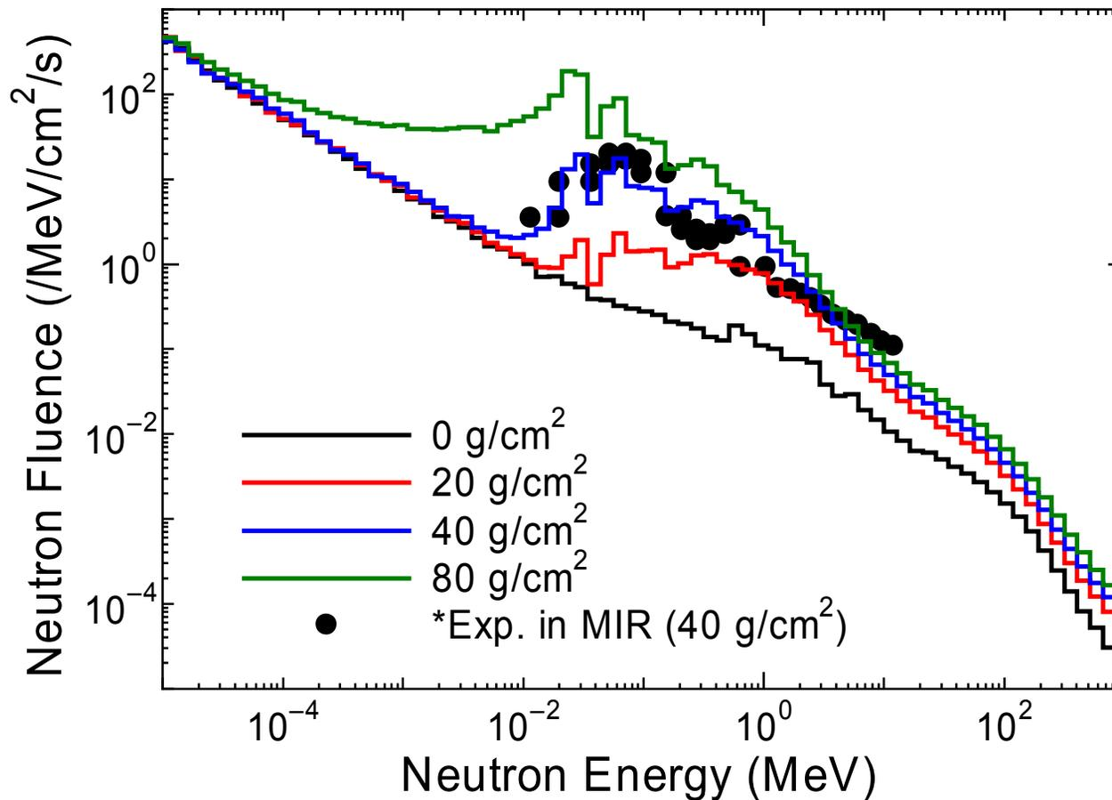
**Neutron Spectra inside Cylindrical Shell**
