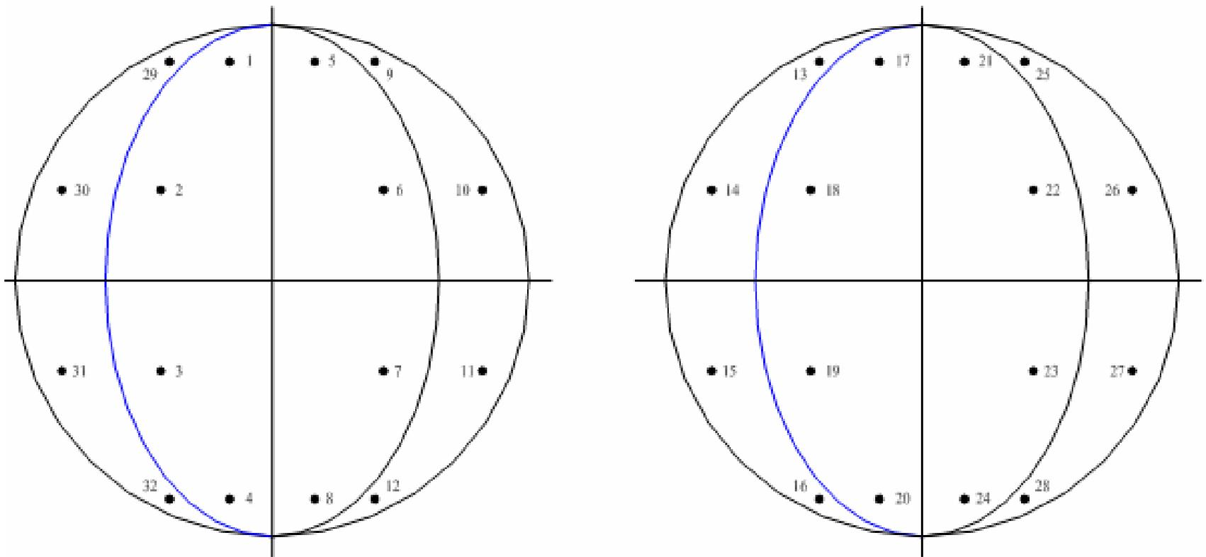
**32 pockets with the detectors on the phantom surface**
