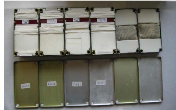
Passive detectors inside the capsule in 4 SPD boxes
