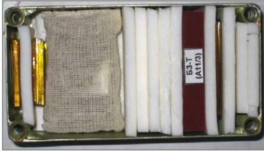
Passive detectors inside the capsule in 4 SPD boxes
