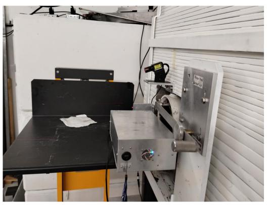
Pb target placed in and out of beam via Al handle.
