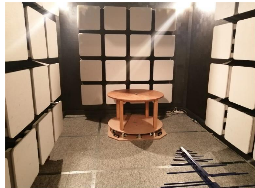
Photo 8.1: Setup for radiated emissions test (30MHz-1GHz)
