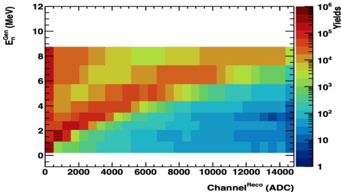
Figure: PTB delivered energies and the measured recoil distribution, 8 monoenergetic runs used.
