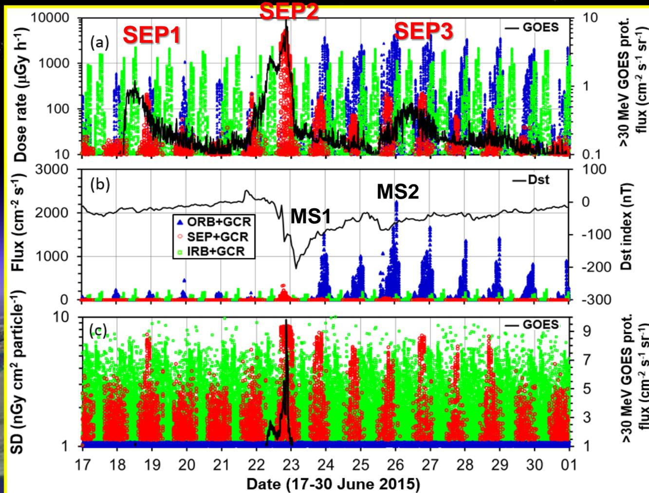
The GCR source is seen in the bottom of the dose rate bars for dose rates below  $20 \mu\text{Gy h}^{-1}$
