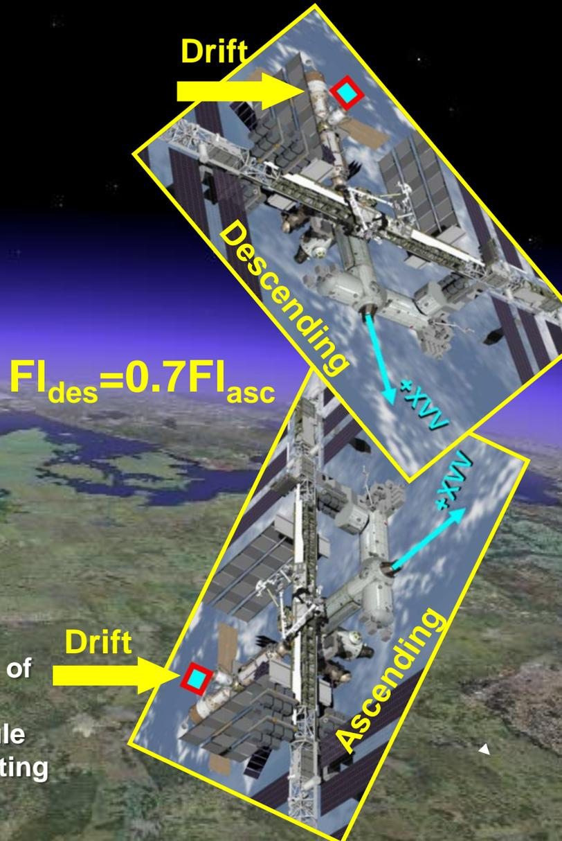
The R3DR2 detector that was located on the left side of the ISS “Zvezda” module against the ISS vector of velocity, was heavier shielded by the “Zvezda” module body on the descending orbits from west to east drifting inner belt protons, when the ISS was in the nominal “+XVV” orientation
