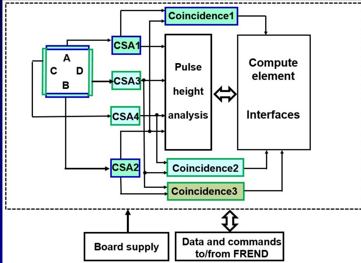
Two dosimetric telescopes (A&B) and (C3&D) in perpendicular directions. Each telescope consists of two Si PIN photodiodes. A coincidence technique for the associated with each dosimetric telescope signals is applied to obtain LET .
