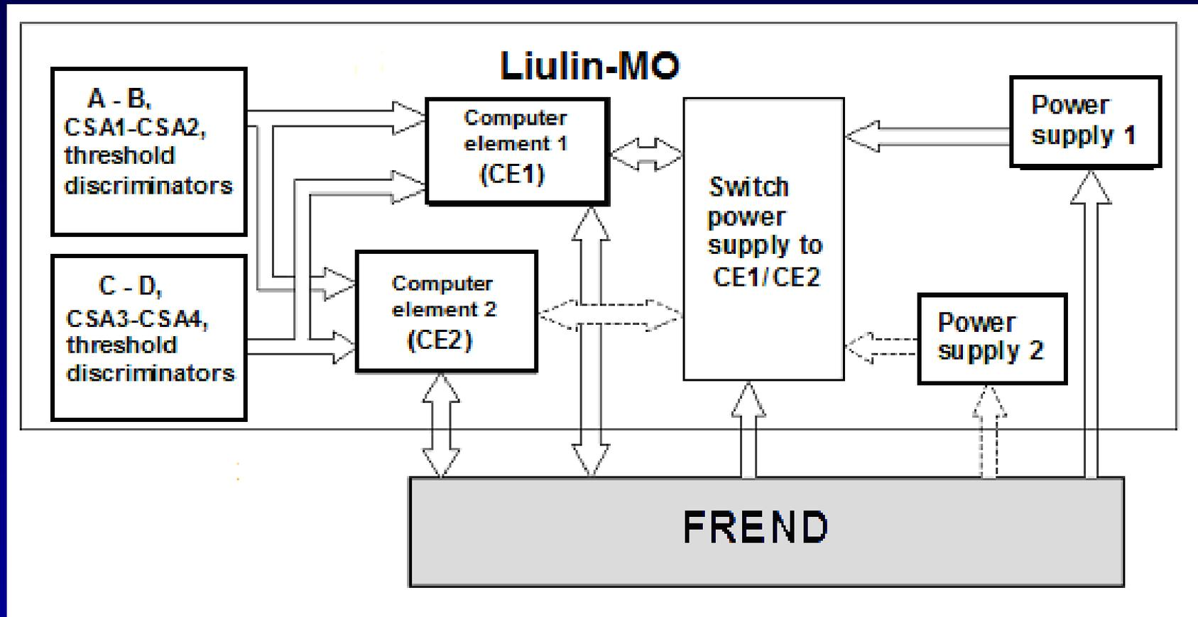
**Nominal and redundant side of the dosimeter**
