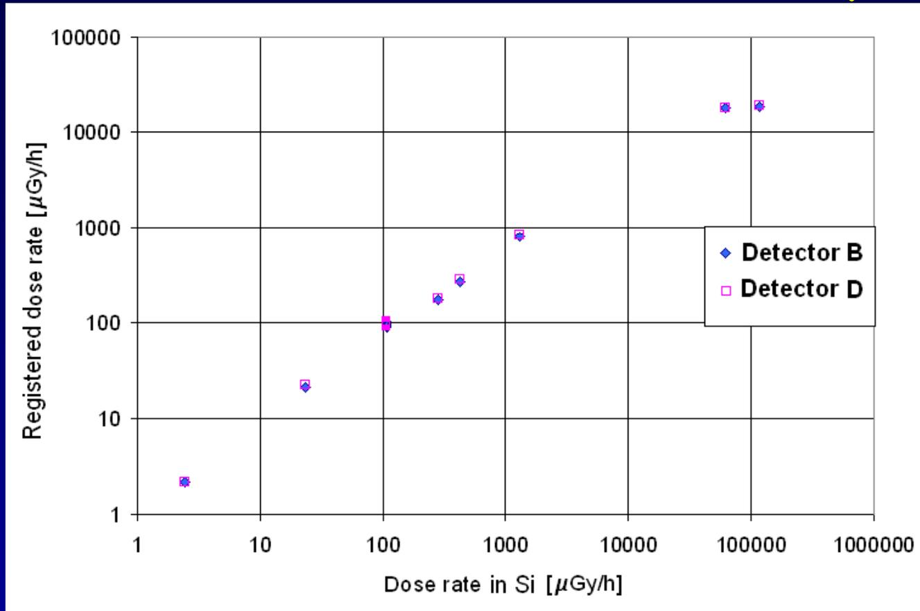
Calibrations at the Research Department of Ionising Radiation Metrology – Russia by means of standard  $^{60}\text{Co}$  and  $^{137}\text{Cs}$  sources.
