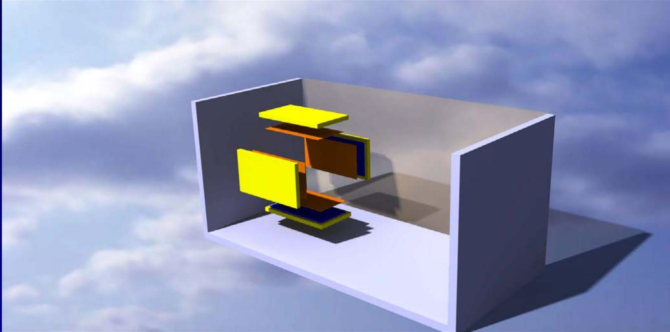
Each pair of the dosimetric telescopes consists of two 300  $\mu\text{m}$  thick, 20x10 mm area rectangular Si PIN photodiodes. The distance between the parallel Si PIN photodiodes is 20.8 mm.
