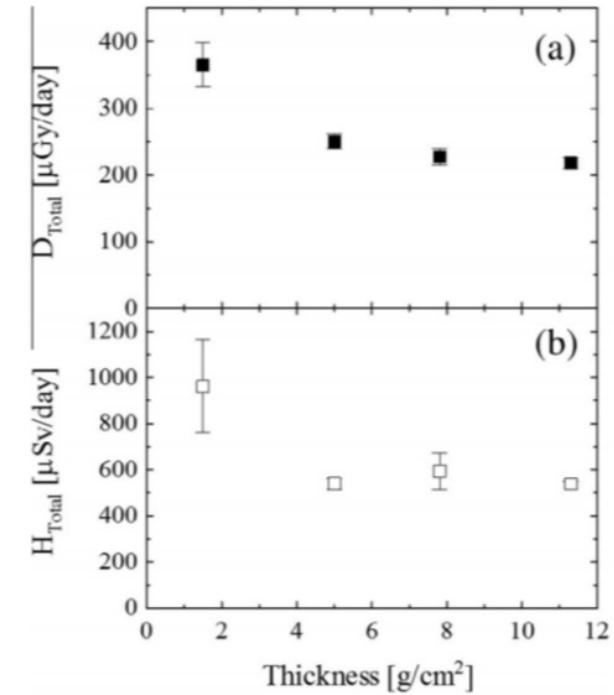
Variations of (a) total absorbed dose ( $D_{Total}$ ) and (b) total dose rate ( $H_{Total}$ ) as a function of the material thickness.
