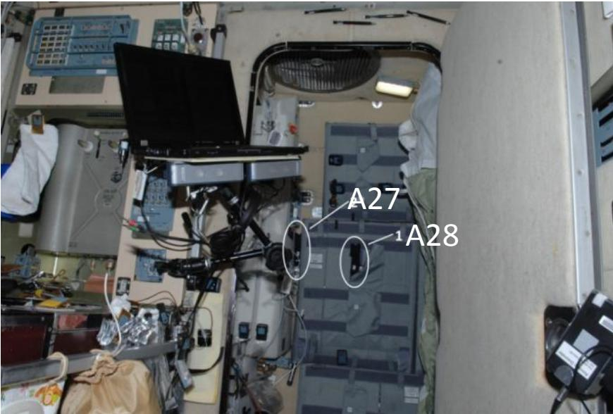
SPND A28 and A27 dose rate for 3 sessions (2010) in detector configuration shown on figure above.
