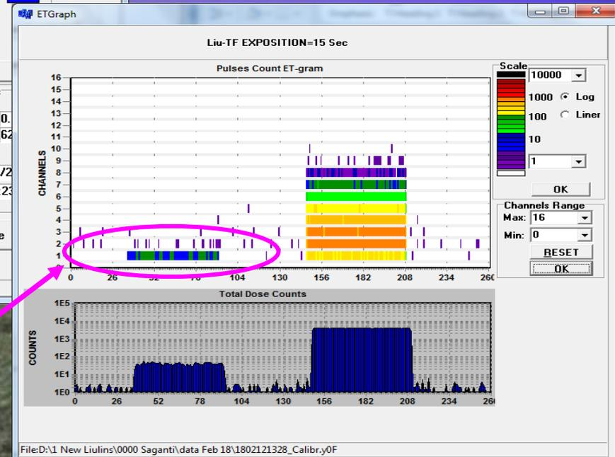
All deposited energies of 60 keV  $^{241}\text{Am}$  gamma line fall into the first channel of the spectrometer having a range from 40 to 80 keV. This proves the correct settings of the 1<sup>st</sup> channel.
