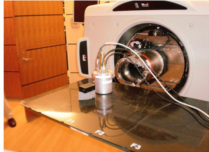
Proton and Carbon Radiotherapy beams possess higher LET and RBE than do x-ray and electron radiotherapy beams...yet ionization chambers are still used in calibration for all of them.
