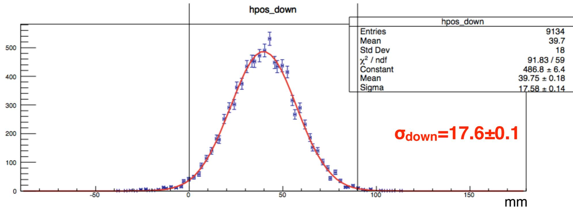
$\sigma_{\text{machine}} \sim 15\text{mm}$  at the isocenter (without any material in between)
