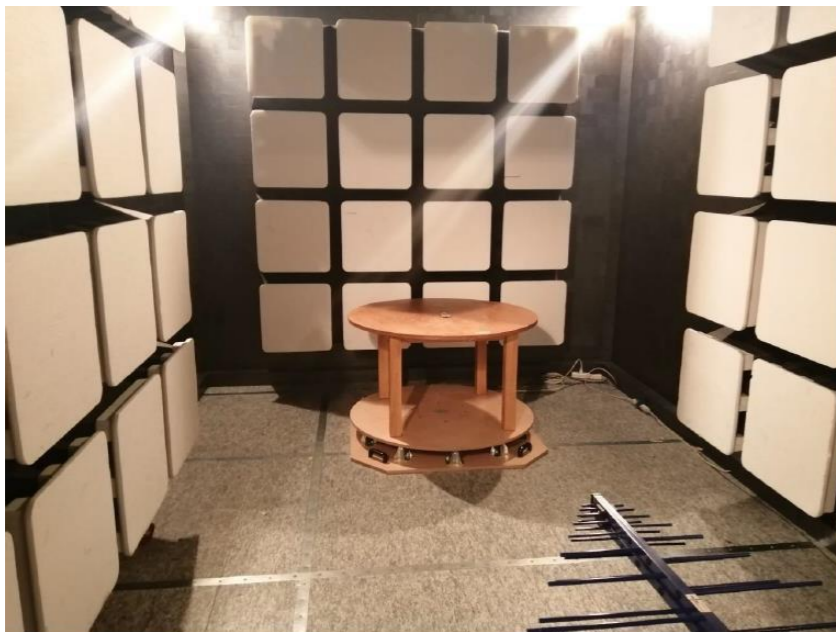
Photo 8.1: Setup for radiated emissions test (30MHz-1GHz)
