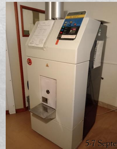
^{137}\text{Cs} Irradiator A=36.67 TBq
