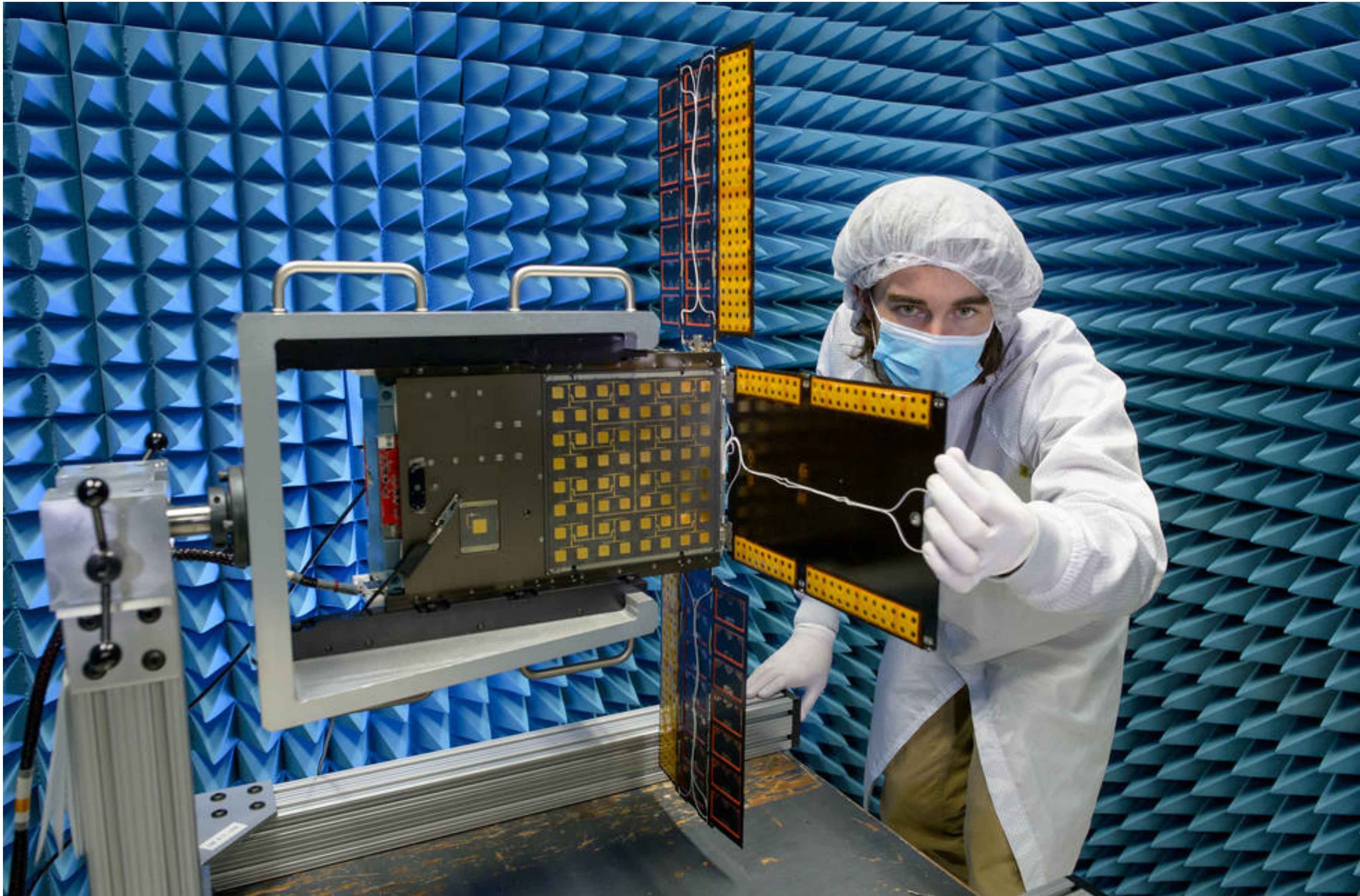
Biosentinel Cubesat EMI Testing
