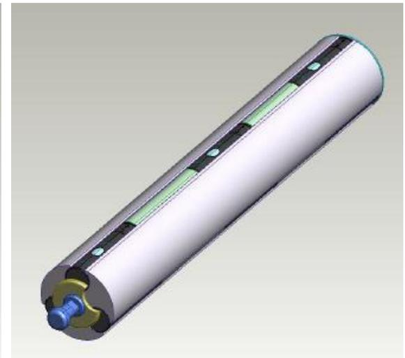
3 – After inserting: cells are fixed after rotating the knob of the holder
