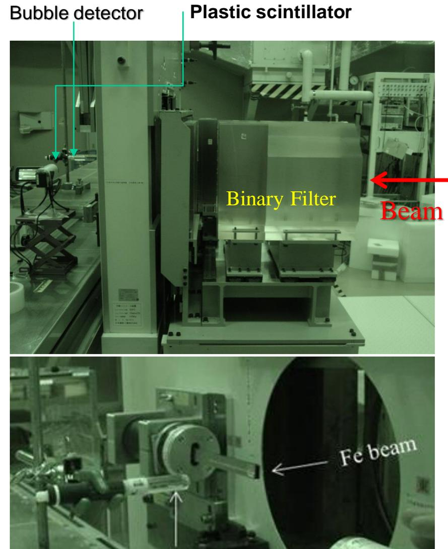
Fig.2: Experimental Setup at HIMAC-NIRS
