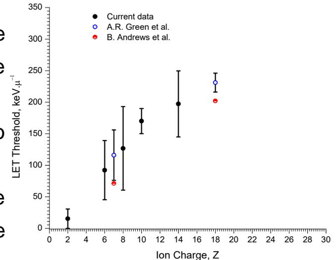
**Fig.10: Z-dependence of LET threshold**
