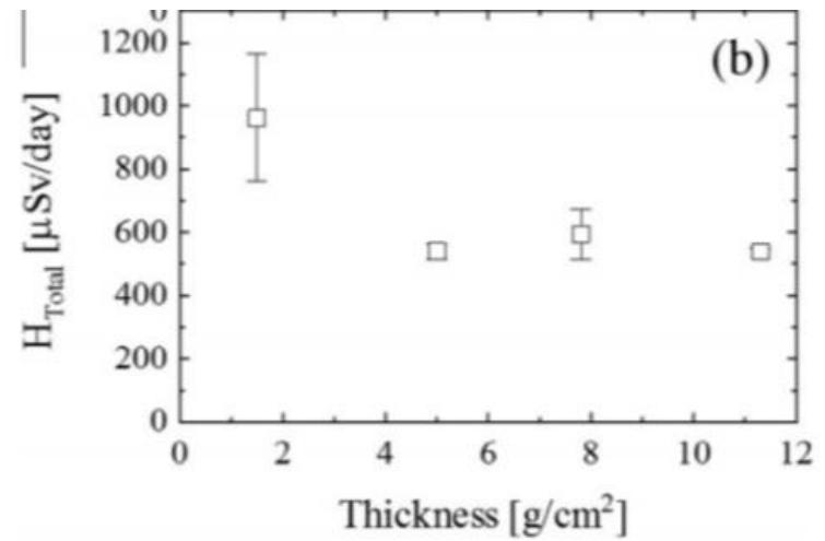
Variations of (a) total absorbed dose ( $D_{Total}$ ) and (b) total dose equivalent ( $H_{Total}$ ) rates as a function of the material thickness.
