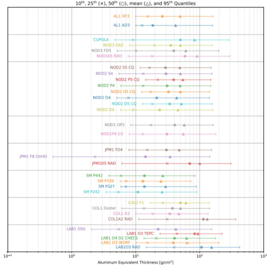
Figure 16: Statistical quantities on shielding thickness (for Aluminium) in various locations across ISS.
