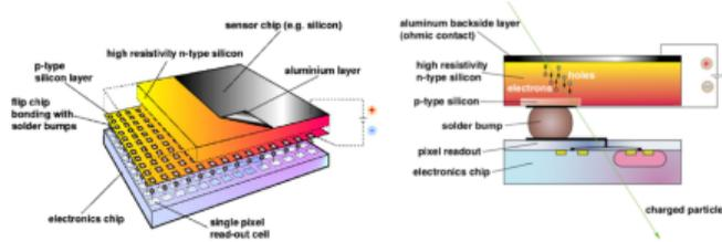
Figure 1: Medipix2 chip and Timepix assembly.
