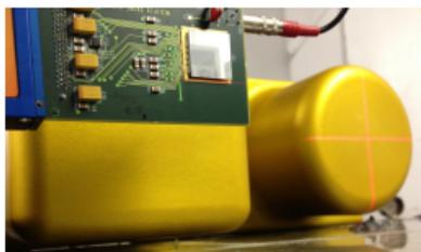
Figure 2: Timepix on carrier board in front of ISS-RAD during  $p^+$  testing in 2014.
