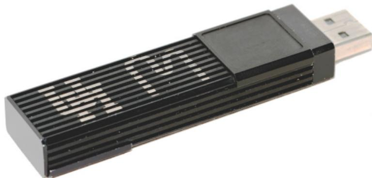
Figure 3: Radiation Environment Monitor.
